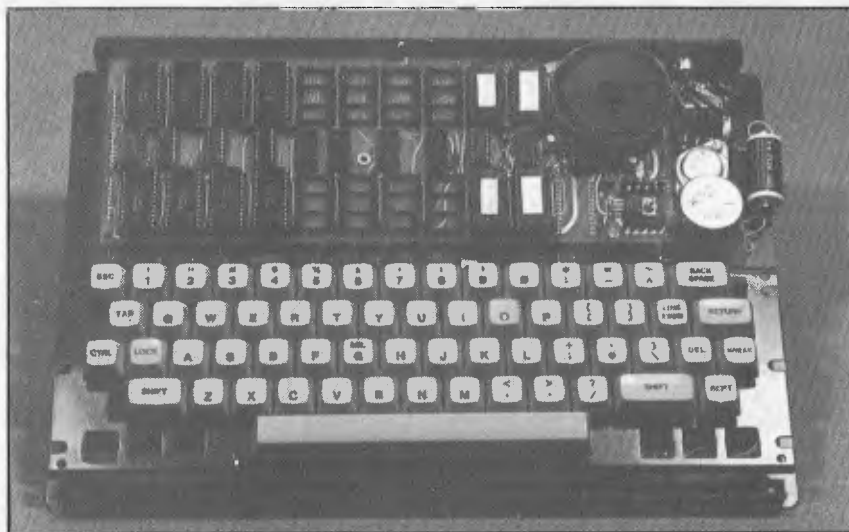
MicroBee with cover removed.
